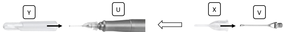
Fig. 6 Exemplary product illustration of putting sleeve and test chamber onto phaco tip
